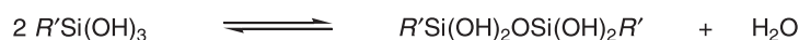
Fig. 3. Key reactions of alkoxysilanes (in the condensation the two silanols are not necessarily identical, one may, e.g. , be a surface-SiOH group)
